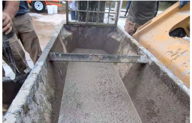
The reversible auger and tighter tolerances between the auger and trough results in superior mixing and dispensing. The 750 Mixer features up to a 3/4-yard capacity.
