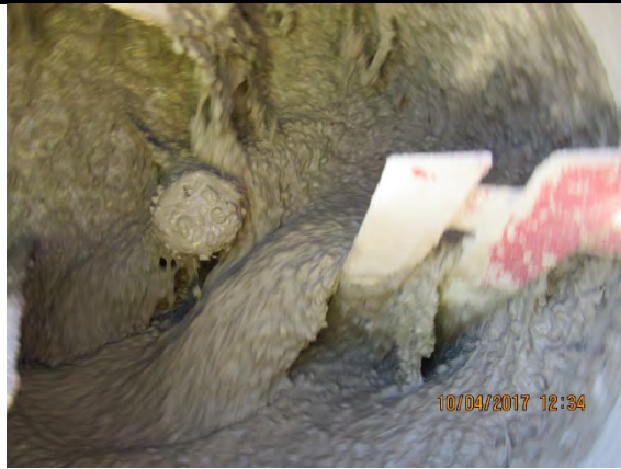
Photograph: 94013 CTS, Rapid Set and Helix Fiber Subject: Mixing of bagged product, aggregate, and fibers
